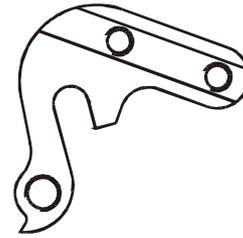
**Fig. 8:** right-hand dropout
